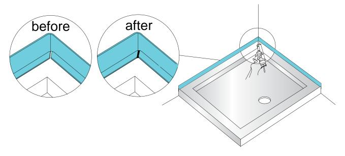
(6) A water barrier has been created and tile can be fixed on wall and down to tray.
