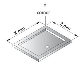
2 Cut tiling bead to required length X + Z, and make two 45° cuts at the position point Y.
