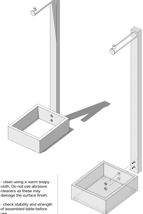
fit and tighten the two allen bolts as shown
