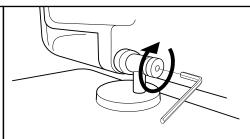
**6.** Use the hexagon key to tighten the hinge pins. Check that the seat and cover are secure before use.
