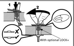
1. Assemble the hinge and gasket and slide the tab and bolt through the pan until it engages on the underside. Finger tighten only. Ensure the tab is the correct way up.
