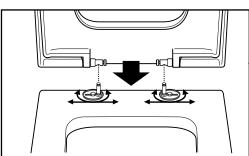
**3.** Lower the seat/cover onto the pan, engaging the hinge pins with the hinge bases. The position of the hinge bases may need to be adjusted to allow this.
