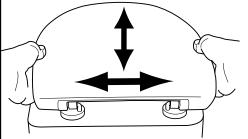
**4.** Adjust the hinges to centralise the seat on the pan and to allow the correct degree of seat/cover overhang at the front.
