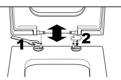
**5.** Once adjusted, remove the seat/cover and tighten the bases with a spanner or screwdriver. Clip the hinge covers in place before replacing the seat/cover. Care should be taken not to overtighten the fixings.
