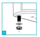
Secure the valve to the cistern by replacing the plastic washer and screwing the nut to the thread. Do not over tighten.
