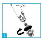
To connect, screw the thread into the sprung loaded opening ensuring this is fully secure but not over tightened
