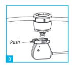
When connecting the button it is very important when deciding on the position that the cable runs smoothly, this prevents valve failure. Once the position of the button is decided fix into position as shown. Please note the hole size for the button in 40mm.
