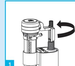
1 Turn off water supply and turn arm anticlockwise. Do not remove cap.
