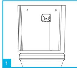
1 Measure the height of the cistern, so the valve can be set to the correct height.
