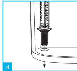
4 Remove the plastic washer and nut from the thread and position the valve in the cistern ensuring the conical rubber seal sits on the hole at the cistern base.
