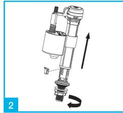
2 To adjust the height remove red plug, turn the valve base clockwise and then adjust height to the correct level
