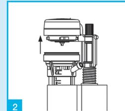
2 Lift the top assembly away from the valve holding the arm.
