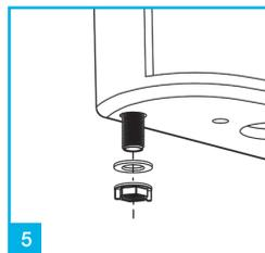
5 Secure valve to the cistern by replacing the plastic washer and screwing the nut to the thread. Do not over tighten.
