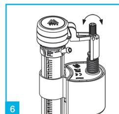
6 The water level can be adjusted by turning the adjustment screw (clockwise for more water, anticlockwise for less water).
