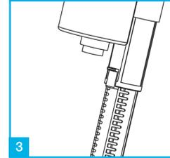
3 Once the correct height is achieved, turn base back anticlockwise and re-insert red plug.
