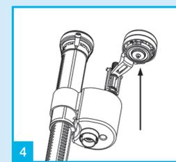
4 Remove diaphragm washer and clean with water or replace.
