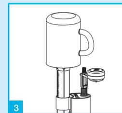
3 Turn water supply on and off to clear any debris. Hold a cup over top to prevent any splashing.
