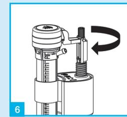
6 Refit top assembly complete with diaphragm and turn on water supply.
