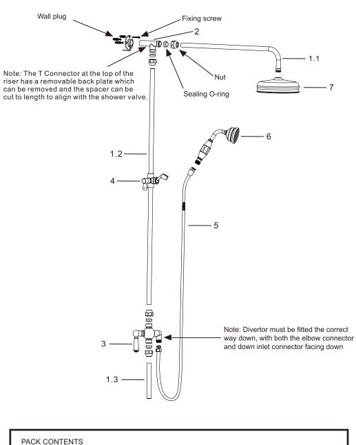
1.1 – Shower arm (Connect Shower head & T connector), 1.2 – Long pipe (Connect T connector & Diverter, add slider handset holder), 1.3 – Short pipe (Connect Diverter & Shower valve), 2 - T Connector (Add Shower arm & Securing bracket, Including 3 x wall plug, 3 x fixing screw and allen key) 3 - Divertor (Add Shower hose & Handset), 4 – Slider handset holder, 5 – 1.5m Shower hose, 6 – Handset, 7 – Shower head
