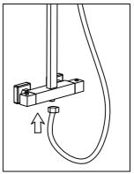
Connect the shower hose to the bottom outlet on the shower valve, and screw the conical end to the shower handset. Place the conical end of the shower flex into the parking bracket on the riser rail.
