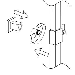
Install the riser into the top outlet of the shower valve.
