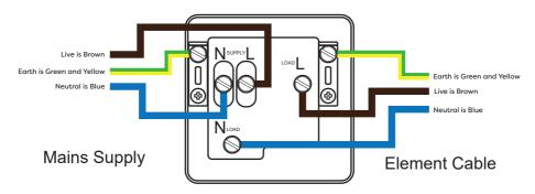
Diagrams are for illustration purposes only. Your switch may superficially differ from this drawing. Refer to the instructions of you chosen switch for guidance is needed
