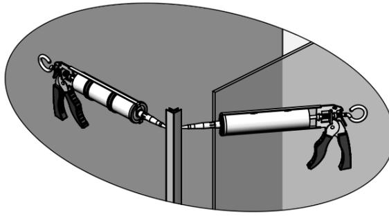
TO FIX THE OPTIONAL GLASS PANEL INTO PLACE, FIRSTLY RUN A SMALL BEAD OF SILICONE DOWN THE INSIDE OF EACH GLASS SLOT ON THE CORNER PROFILE (ITEM 15) STOPPING 5mm SHORT AT EITHER END.
