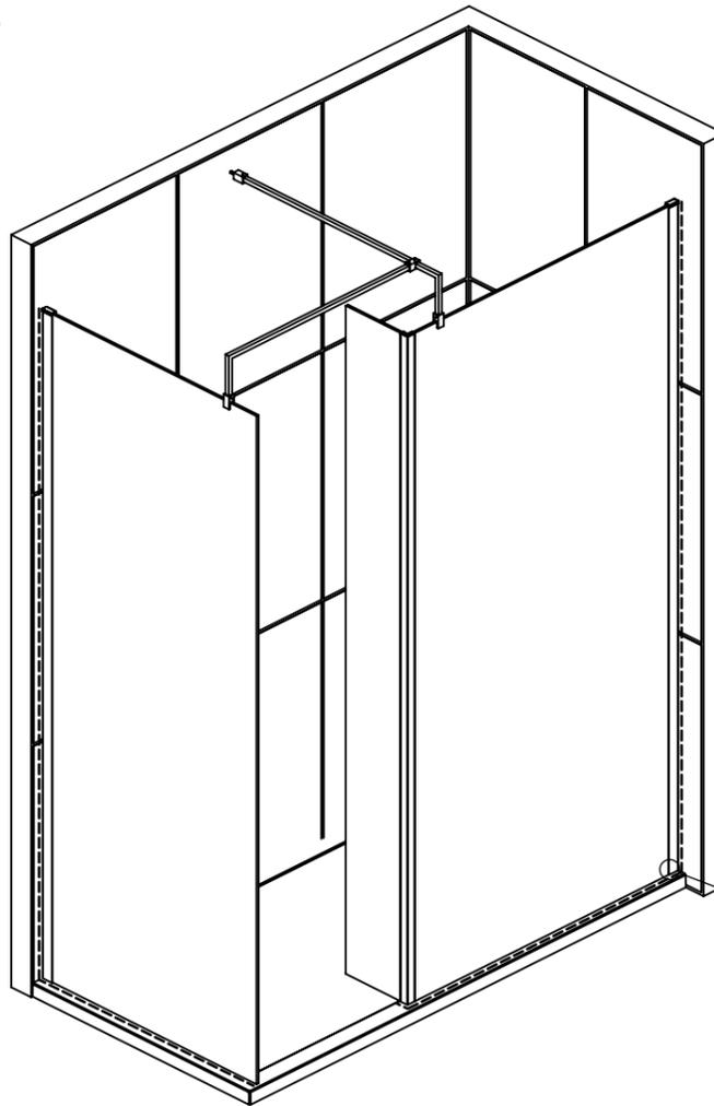
EXTERNALLY SILICONE SEAL THE WALL PROFILE WHERE IT MEETS THE WALL AND ALONG THE BOTTOM OF THE GLASS. ALL IN A CONTINUOUS BEAD.
