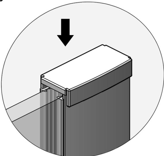
FIT THE WALL PROFILE CAP(S) (ITEM 4). A SMALL BLOB OF SILICONE CAN BE APPLIED TO THE UNDERSIDE OF THE CAP TO HOLD IT IN PLACE IF NECESSARY.
