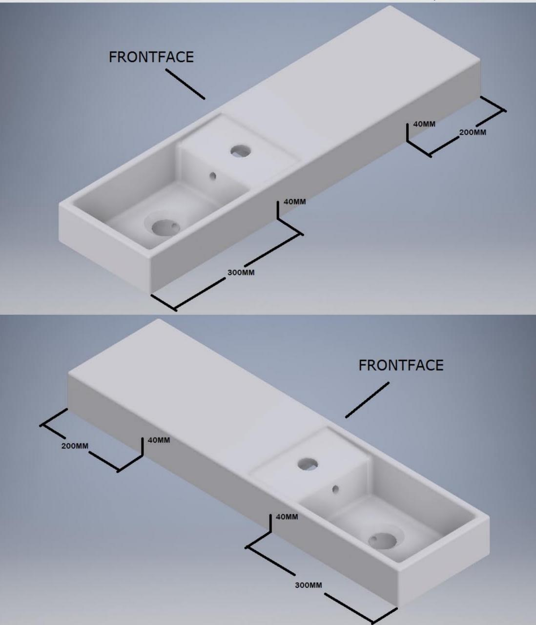
On the back face of the basin measure 300mm in from the bowl side and 40mm up from the bottom. On the opposite edge mearure 200mm in and 40mm up (as shown in the diagram above)
