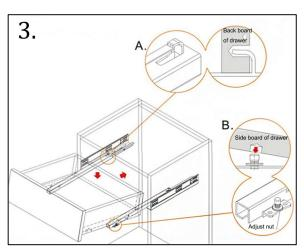
Adjust nut B: Fine turing the front panel up/down
