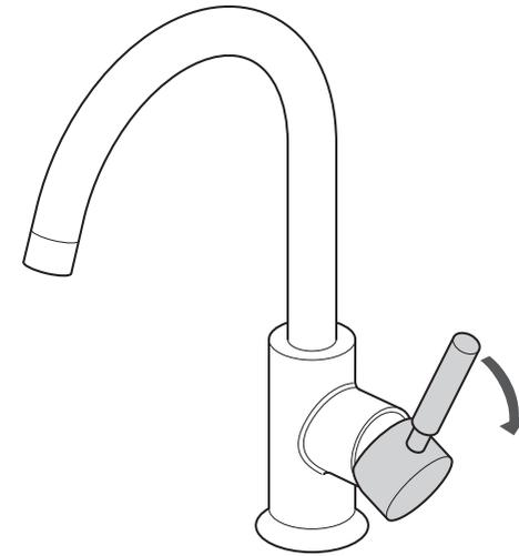
Moving the mixer lever to the right will increase the flow of water.
