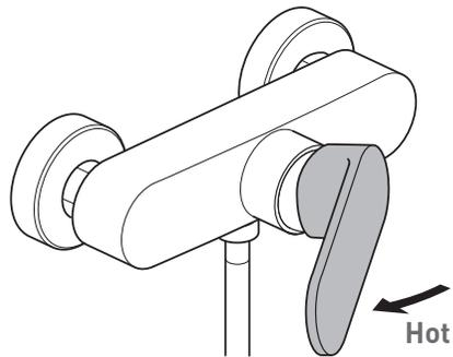
Moving the mixer lever from right to left will increase the water temperature.
