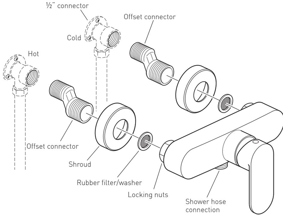
Before installing your new mixer, flush through the pipe work to ensure removal of debris, turn off the water supply.
