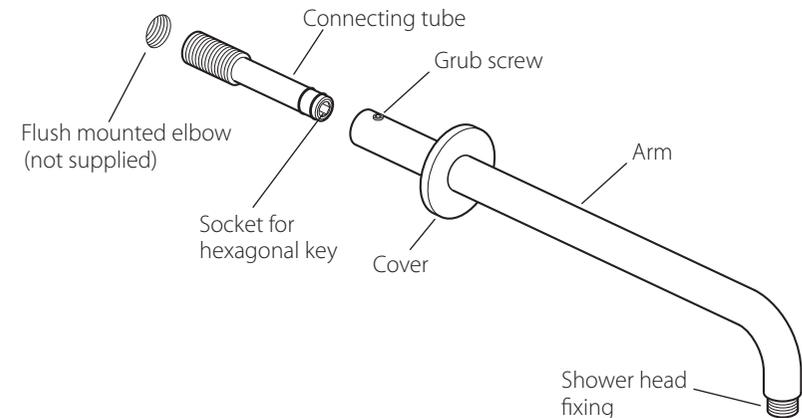
Prepare the end of the pipe work with an 1/2" fixed elbow (not supplied). Fix in the correct position, and flush with the final surface of the wall.
