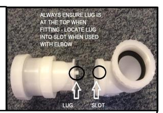
INSTRUCTIONS - REMOVE ELBOW TO USE AS INLINE TRAP. REMOVE PLASTIC BUSH FROM ELBOW FOR 1 ½ THREADS. SELECT APPROPRIATE BLACK WASHER FOR RELEVANT SIZE OF WASTE PIPE. IMPORTANT: ALWAYS POSITION LUG AT THE TOP OF FITTING. DO NOT TOUCH INTERNAL RUBBER MEMBRANE WITH FINGERS OR OTHER OBJECTS.
