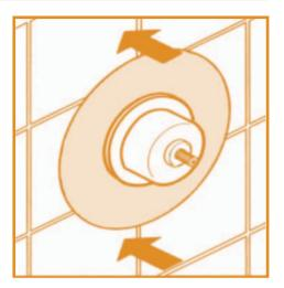
• Place Grommet within the concealing plate centre and push the plate into position
