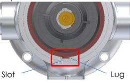
Place the new cartridge in the valve as in the diagram.
