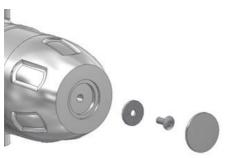
NB - Please make sure the valve is isolated from the water supply before replacing a cartridge. When the valve has been isolated, turn on the valve to let any water in the pipework escape.
