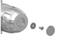
Turn the handle clockwise until it stops in the off position. Remove the cap and undo the screw. Remove the screw and washer. Put these in a safe place. The handle can now be removed.
