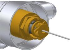
In order to calibrate the valve to the correct outlet temperature please place a 3mm flat bladed screw driver into the spindle. Locate the calibration screw slot inside and turn anticlockwise to increase the temperature or clockwise to reduce it. Allow the valve to stabilise after every adjustment and measure the outlet temperature.
