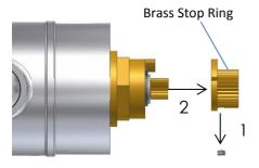
Please remove the M4 grub screw from the Brass Stop Ring. The Brass stop Ring can then be removed.
