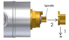
In order to stop the flow of water the Brass stop Ring position must be reset. To do this, remove the M4 grub screw holding the Brass Stop Ring in position. Then remove the Brass stop Ring.
