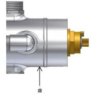
Tighten the chrome retaining collar by turning it clockwise. Tighten the collar to 17 Nm and then replace the grub screw to ensure the collar does not come loose.
