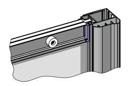
IF THE ENCLOSURE OR SIDE PANEL HAS THE OPTIONAL SCREW COVER PROFILES (ITEM 2) PUSH FIT THEM ONTO THE SCREW COVER PROFILE FIXING CLIPS (ITEM 3).
