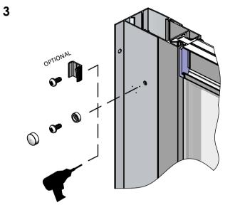
WHEN THE ENCLOSURE IS READY TO BE FIXED, DRILL THROUGH THE HOLES IN THE WALL PROFILE AND CORNER POST WITH A 3mm DRILL. (MAKE SURE YOU ONLY DRILL THROUGH ONE WALL THICKNESS) THEN FIX THE FRAME WITH ITEMS 10, 11\* & 12\*.
