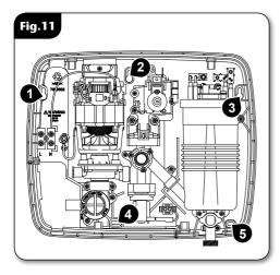
After choosing the site for the shower, use the backplate as a template **(fig.11)** and mark the four fixing holes 1, 3, 4 and 5.
