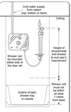
Fig.5 Diagrammatic view (not to scale)
