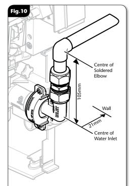
Note: If installing a feed pipe from the back, the use of a soldered Elbow connector is recommended. It should be positioned approximately 105mm from the inlet connector centre. The centre of the inlet valve to the wall surface is 21mm.
