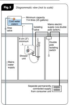
Important: To comply with BEAB care mark in service testing procedure the isolating valve should be located close to the shower unit.
