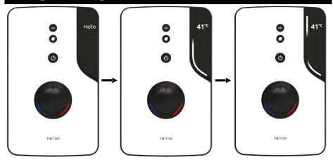
The showering water temperature is shown on the display. The Light Bar gradually fills up, and becomes completely filled after 5 minutes. An animation occurs on the Light Bar, repeating and increasingly more frequent as time elapses. After 20 minutes (by default), the shower will automatically enter Phased Shut Down.
