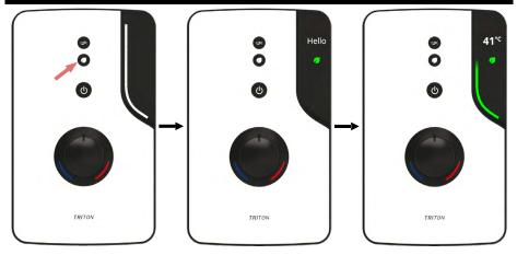
Press the ECO button from Standby to start the shower in ECO Mode. The Light Bar will count down for 5 minutes (by default), after which the shower will automatically enter Phased Shut Down. ECO Mode can be cancelled by pressing the ECO button; the regular timer settings will apply.
