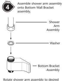
position then tighten bottom nut of lower shower arm to lock in position.
