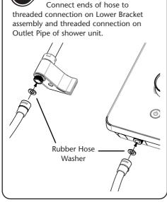
Fit rubber hose washers into cones at both ends of hose.
