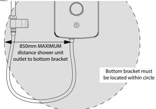
b) The kit can be installation in both left hand and right hand corner installations. It can also be installed at any intermediate position along a wall, in both left hand and right hand orientations
