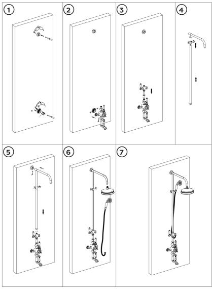
**ATTENTION:** Having first checked all new connections, close all taps except the new mixer and as system starts to refill, check for leaks. Once you have satisfied yourself that there are no leaks. Turn on the hot+cold water supplies.
