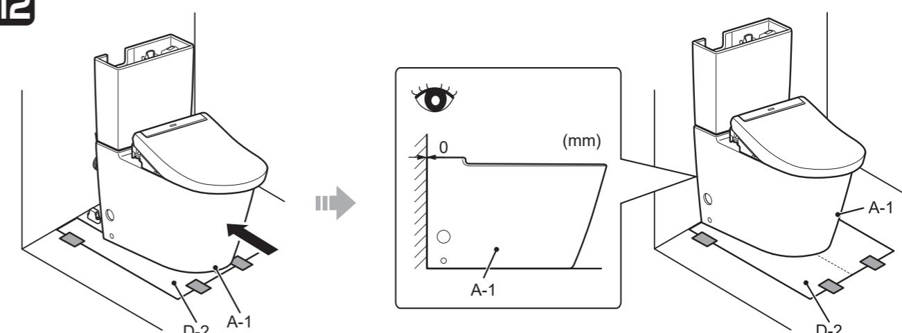
\*If there is a water supply hose and power supply cable for a main unit, make sure they are not pinched between A-1 and the wall.
