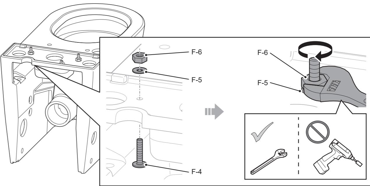
\*Be careful not to over-tighten, as doing so could damage the porcelain. /
