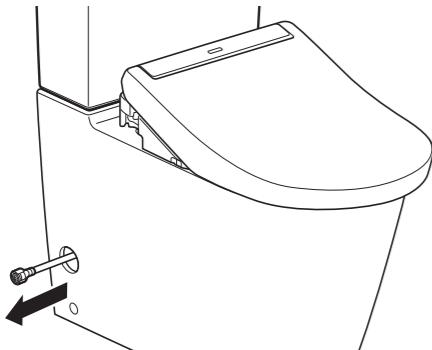
If the shutoff valve is on the right side, pull the water supply hose out from the right side. /
