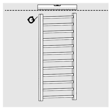
Allow enough room for the installation of valves or thermostatic controls.
