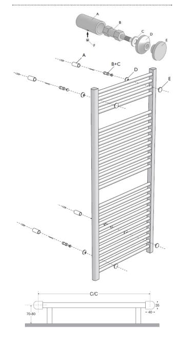
Tapping centres (C/C) for Hugo2 radiators are 40mm less that the width of the rail and 70mm out from the wall
