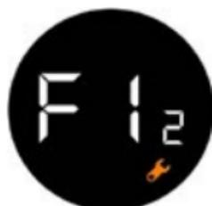
The Radiator Valve will close the valve at a specific time, and then open it again to detect the exact opening position of the valve. The automatic detection function will make the radiator valve as efficient as possible and will control the temperature more accurately.
