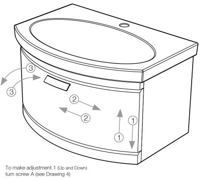
To make adjustment 2 (Left and Right) turn screw B (see Drawing 4)
