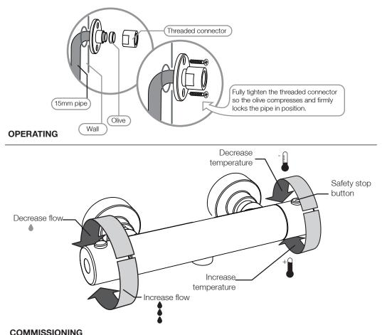
It is important that incoming water supplies conform to the requirements specified for pressure and temperature. Assure that supply water conditions satisfy any guidance information for the control of bacteria and that the designation of the supplied valve suits the application. Do not continue commissioning until supplies are correct and stable considering variation caused by other service users.
