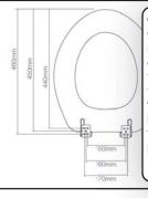
4. Compare the measurements of the toilet pan to the toilet seat to determine which fixing holes to use on the hinge plates.
