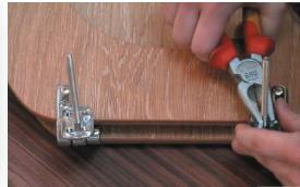
When using pliers grip as close to the hinge plate as possible. As this part of the thread is redundant and won't affect the wing nut.
