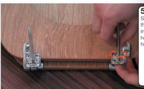
5. Screw the threaded bars into the chosen holes on the hinge plates.
