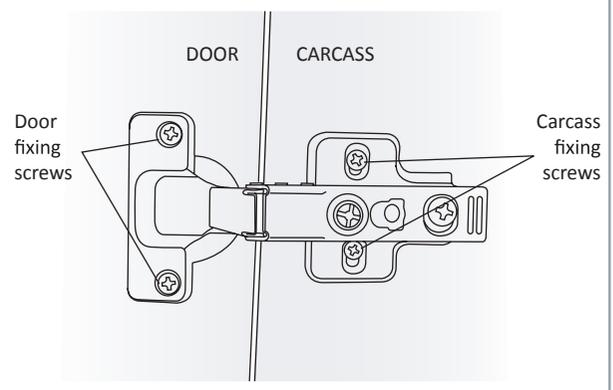
Choose the desired handing and fix hinges to the door and then the carcass. Holes are also provided on both ends of the door for the badge attachment to be fitted once the desired hinge position is chosen.
