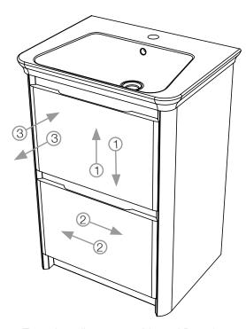
To make adjustment 1 (Up and Down) turn screw A (see Drawing 2)
