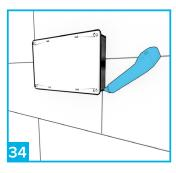
Cut and discard the corrugated part of the cover with a knife, flush with the finished wall tiles.
