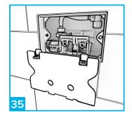
Remove inspection cover and turn on the water, using the isolation valve inside.
