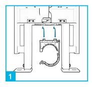
Insert the drain connector clip into the frame and slide to the left to lock into position. The clip can be flipped 180° to suit the pipework.
