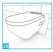
Place the pan onto the bolts. Ensuring someone is holding it into position check tha pan is level.
