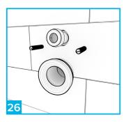
At this point lubricate the cut ends and insert the connectors fully into the corresponding wall outlets.
