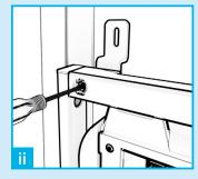
Locate the wall fixing brackets, offer them up behind the frame and using a phillips screw driver, screw the bolt into the bracket 2-3 full rotations.
