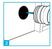
Insert the supplied drain connector into the soil pipe. *Optional angled drain connectors are available for connection to floor outlets.*
