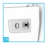
Secure on both sides with plastic washer, metal washer and nut. Please note depending on the brand of pan fixing method may differ.
