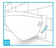
Cut the wall membrane around the outer edge of the toilet and discard the excess membrane
