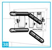
Depending on the depth of your wall, the central button rods may need breaking off before inserting.
