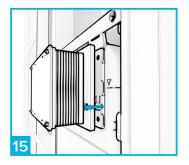
Attach the cover over the inspection plate to prevent debri getting into the cistern.
