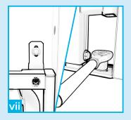
Place the frame back between the joists, and using a socket wrench or spanner secure to the wall and floor using the supplied screws.
