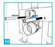
Insert the toilet hanging threads, using whichever hole combination corresponds with the toilet hanging holes (180mm/230mm). Then slot the sheaths over the theads.
