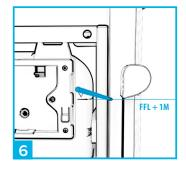
Measure up from the FFL 1m and mark on the joist. Raise the frame so that the recommended 1m indicator on the frame lines up with the 1m marking on the joist.
