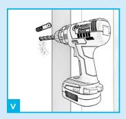
Remove frame and place to one side. Drill two 10mm holes where marked on the wall, and insert the supplied raw plugs.
