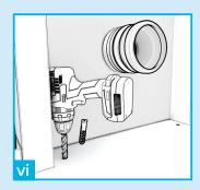
Drill two 10mm holes where marked on the sub-floor, and insert the supplied raw plugs.
