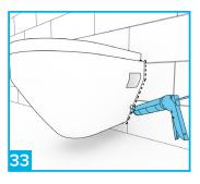
Once you are happy there is no leaks seal the rear edge of the toillet with silicone sealant.
