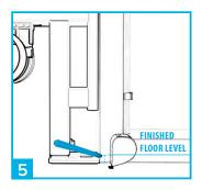
Measure from the sub floor and mark on a joist the height of the intended finished floor level.
