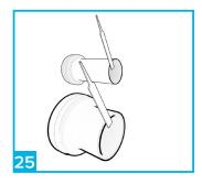
File a small chamfer onto the outer edge of the cut ends of the connectors. Ensure they are smooth to the touch.
