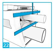
Locate the pan connector and flush pipe connector. Insert onto the rear of the toilet and mark a line on each, level with the back edge of the toilet.
