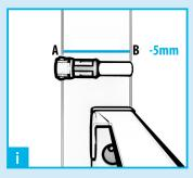
Locate the wall fixing bolts. Measure and cut the bolts using a hacksaw 5mm shorter than the total depth of the wall void. Then clip the bolts into the top frame adjustment holes.
