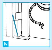
Ensuring that the feet of the frame are flush with the front edge of the joists, mark on the sub-floor the locations to be drilled.
