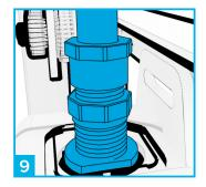
Connect the water supply to the 1/2" thread near the top right hand side of the cistern.
