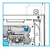
Ensure that the isolation valve is closed by twisting it fully to the right.
