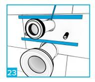
Remove the connectors from the toilet and insert fully into the corresponding wall outlets. Mark a line flush with the finished tiles.
