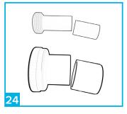
Measure the gap between the two lines, and cut off the same distance from the end of the connecors. (We would reccomend removing a further 3mm)
