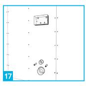
Cover the stud wall with plasterboard, cutting holes for the button opening, flush pipe and pan connector outlet.
