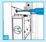
To ensure the frame is plumb, adjust the level of the frame using the adjustment bolts.
