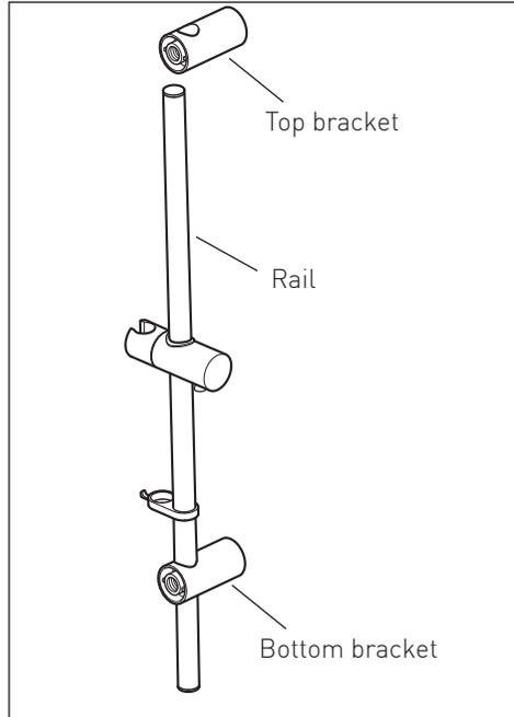
Push a rubber insert into the hole of the bracket, screw in the grub screw and tighten.
