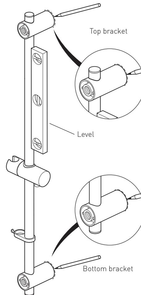
Find the centre of the marked position. Suitably fix the wall bracket to the wall using appropriate fixings.
