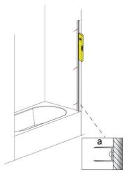
Remove wall channel from the side panel frame. Place wall channel in position on the Bath (20~22mm in from the edge of the bath), use a spirit level to ensure that it is vertical and mark all 3 fixing holes onto the wall.
