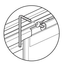
If the door is not square with the fixed panel or doesn't close correctly, one or both of the top sliders should be adjusted.
