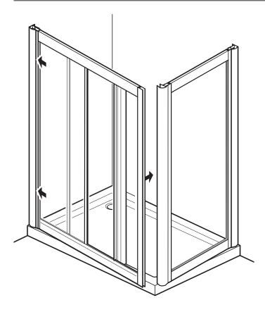
Insert the door into the other wall channel and swing the free end into position on the tray. Push the corner post, fixed to the side panel, onto the side of the door.
