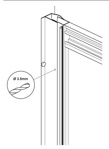
Fix the door to the wall channels. From inside, drill 3 holes through each wall channel (in the marked positions) into the door frame using a 3.5mm drill bit. Fix using 6 x 10mm screws (A) and push on the screw covers (D).
