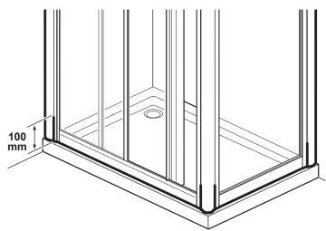
**Sealing outside:** Run a line of silicone sealant from top to bottom down the joint between the wall channels and tiles. Run a line of silicone sealant 100mm up the joint where the door and side panel slot into the wall channels and corner post. Run a line of sealant around the base in the joint between the bottom of the enclosure and the tray, from wall to wall.
