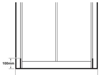
**Sealing outside:** Run a line of silicone sealant from top to bottom down the joint between the wall channels and tiles. Run a line of silicone sealant 100mm up the joint where the door slots into the wall channels. Run a line of sealant along the base in the joint between the bottom of the enclosure and the tray, from wall to wall.
