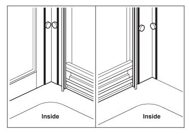
Before sealing you must make sure that the door opens and closes correctly.
