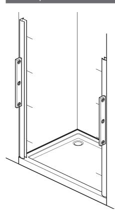
Remove both wall channels from the door frame. Place each wall channel in position on the tray (10 - 15mm in from the outer edge of the tray), use a spirit level to ensure they are vertical and mark all 8 fixing holes onto the walls (holes inside).
