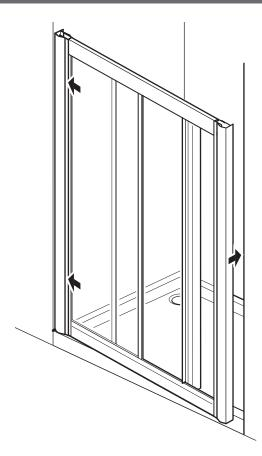
Push the remaining wall channel back onto the door frame on the opening/handle side of the door.
