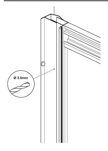
Fix the door to the wall channels. From inside, drill 3 holes through each wall channel (in the marked positions) into the door frame using a 3.5mm drill bit. Fix using 6 x 10mm screws (A) and push on the screw covers (D).
