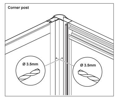
**Note:** Stop drilling as soon as you feel the drill break through the first 2 layers of aluminium. Fix using 6 x 10mm screws (A) and push on the screw covers (D).
