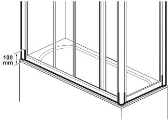
**Sealing outside:** Run a line of silicone sealant from top to bottom down the joint between the wall channels and tiles. Run a line of silicone sealant 100mm up the joint where the door and end panel slots into the wall channels and corner post. Run a line of sealant around the base in the joint between the bottom of the enclosure and the bath, from wall to wall.
