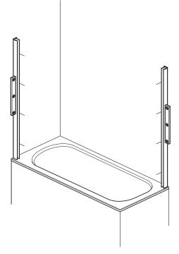
Remove both wall channels from the door frame. Place each wall channel in position on the bath (10 - 15mm in from the outer edges of the bath), use a spirit level to ensure they are vertical and mark all 8 fixing holes onto the walls (holes inside).
