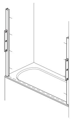
Remove both wall channels from the door frame. Place each wall channel in position on the bath (10 - 15mm in from the outer edge of the bath), use a spirit level to ensure they are vertical and mark all 8 fixing holes onto the walls (holes inside).
