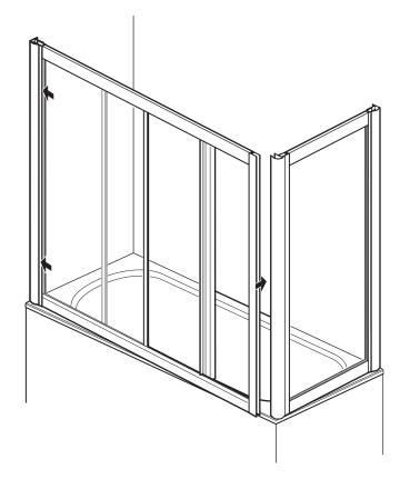
Insert the door into the other wall channel and swing the free end into position on the bath. Push the corner post, fixed to the end panel, onto the side of the door.
