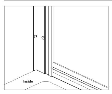
**Sealing inside:** Run a line of silicone sealant from top to bottom down the joint between the wall channels and tiles, also down the joint where the door slots into the wall channels.
