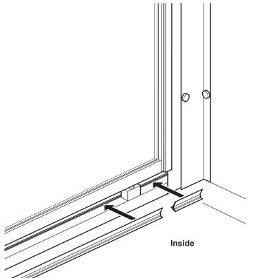
**Optional:** It is only necessary to fit the plastic Anti splash strip (E) if water splashes out through the gap under the door. Cut the strip to size (using scissors) and push fit onto the lug shown on the bottom door frame as shown. *Note: If the anti splash strip catches on the door, simply trim to fit.*
