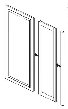
Push the remaining wall channel onto the flat side of the inline panel, then fully push the other side of the inline panel onto the opening/handle side of the door.
