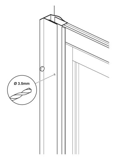
Once you have checked that the door opens and closes correctly fix the door to the wall channels.
