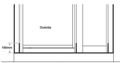
Sealing outside: Run a line of silicone sealant from top to bottom down the joint
