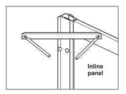
Drill a hole in the position marked on the wall using a 6mm masonry drill bit. Insert a wall plug (C) into the hole (beyond the thickness of the tile). Drill a 3.5mm hole in the position marked on the inline panel. *Note:* Stop drilling as soon as you feel the drill break through the first layer
