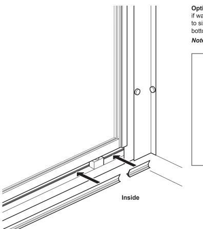
**Optional:** It is only necessary to fit the plastic Anti splash strip (E) if water splashes out through the gap under the door. Cut the strip to size (using scissors) and push fit onto the lug shown on the bottom door frame as shown.
