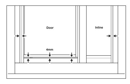
Centre the door/inline panel between the wall channels.
