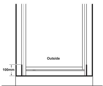
**Sealing outside:** Run a line of silicone sealant from top to bottom down the joint between the wall channels and tiles. Run a line of silicone sealant 100mm up the joint where the door slots into the wall channels. Run a line of sealant along the base in the joint between the bottom of the enclosure and the tray, from wall to wall.
