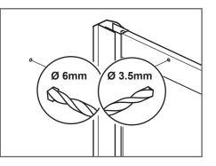
of aluminium. Fix the brace bar to the wall using a 38mm counter sunk screw (I). **Note:** Inject silicone sealant into the hole before inserting the screw to seal the hole. Fix to the inline panel using a 15mm counter sunk screw (H).
