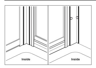
**Sealing inside:** Run a line of silicone sealant from top to bottom down the joint between the wall channels and tiles. Run a line of silicone sealant from top to bottom down the joint where the door and side panel slot into the wall channels and the door slots into the centre post.
