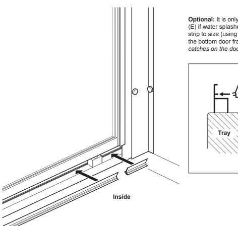
Optional: It is only necessary to fit the plastic Anti splash strip (E) if water splashes out through the gap under the door. Cut the strip to size (using scissors) and push fit onto the lug shown on the bottom door frame as shown. Note: If the anti splash strip catches on the door, simply trim to fit.
