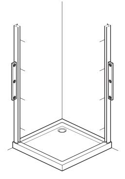
Remove both wall channels from the door frame. Place each wall channel in position on the tray (10 - 15mm in from the outer edges of the tray), use a spirit level to ensure they are vertical and mark all 8 fixing holes onto the walls (holes inside).
