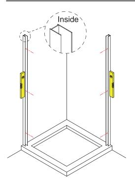
Remove both wall channels from the glass panel frame. **Note:** *Ensure the longer leg of each wall channel is on the inside of the enclosure when fixing.* Place each wall channel in position on the tray (10 - 15mm in from the outer edge of the tray), use a spirit level to ensure that they are vertical and mark all 6 fixing holes onto the wall.
