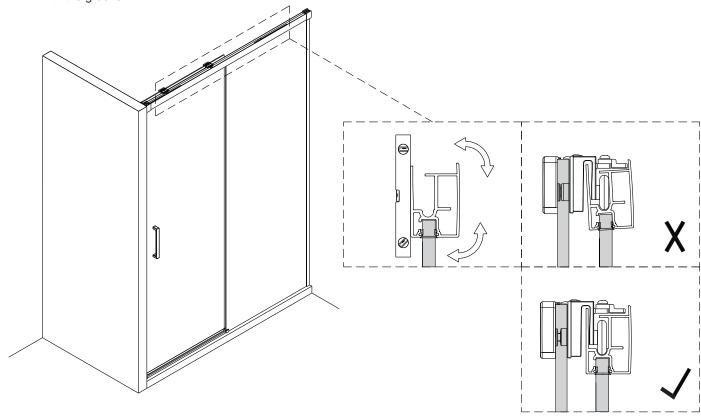
Step 18-4: Tighten the screws at both ends.
