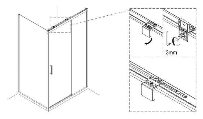
Step 16-2: Loosen the screws at both ends of the roller track slightly.
