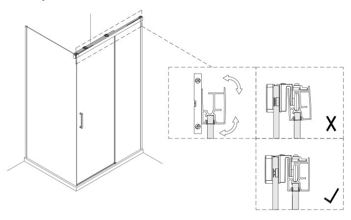
Step 16-4: Tighten the screws at both ends.
