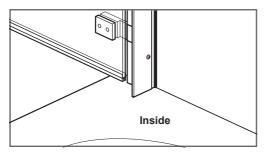
**Sealing:** On the inside and outside, run a line of silicone sealant from top to bottom down the joint between the wall channel and tiles.
