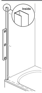
The bath screen should be positioned centrally or slightly toward the inside of the bath rim, as shown. Place the wall channel in position on the bath and against the wall, use a spirit level to ensure it is vertical and mark all 3 fixing holes onto the walls.
