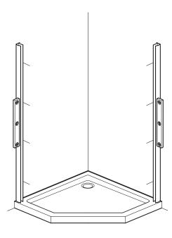
Remove both wall channels from the door frame. Place each wall channel in position on the tray (10 - 15mm in from the outer edges of the tray), use a spirit level to ensure they are vertical and mark all 8 fixing holes onto the walls (holes inside).
