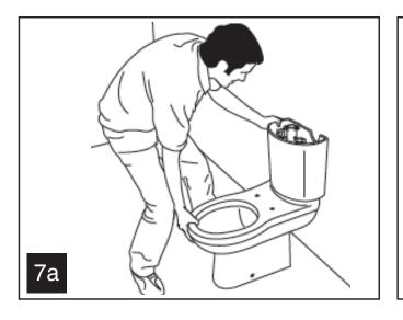
Position the close-coupled pan in the desired location against the wall and align with water supply and outlet connections. If required consult a plumber to ensure correct fixing and to prevent leaks after installation.
