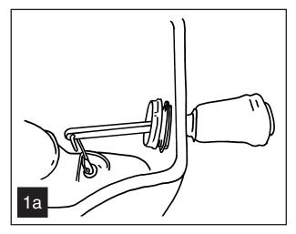
Side Lever Pass the lever through the hole in the cistern Slide the siphon link through the hole in the lever Tighten the nut to secure ensuring parrallel
