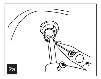
Remove the split pin and washer from the assembly using pliers
