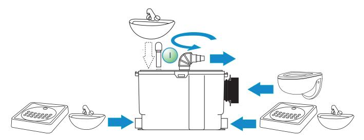
The Sanipack will pump away the waste from a WC, washbasin and shower. Sanipack is for domestic use. Installed and used correctly, Sanipack will give consistent and reliable service.
