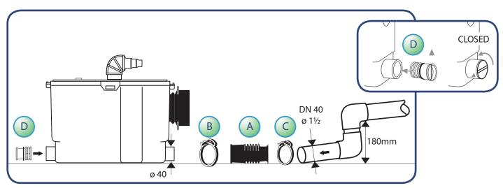
To make the connection to the side inlets, use connector (A). Secure it with plastic clips (B) and (C).
