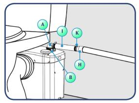
Insert the discharge elbow (A) into the rubber discharge pipe which raises up through the lid, turn to the desired direction and secure with the metal hose clip provided (32-50mm) (B). Then connect the hose to it using the 20-32mm metal hose clip (K), making sure the hose is not kinked.
