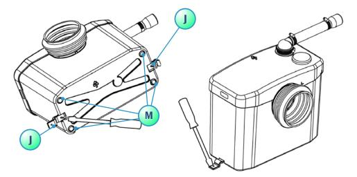
**WARNING:** The unit must be connected to WC pan with a horizontal outlet spigot conforming to EN33 or EN 37. The unit should be accessible for possible service.
