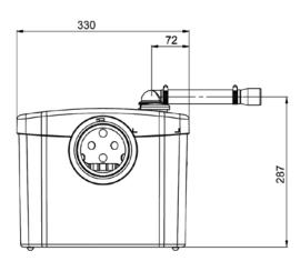
This pump/macerator has been designed to pump away the waste from a WC.
