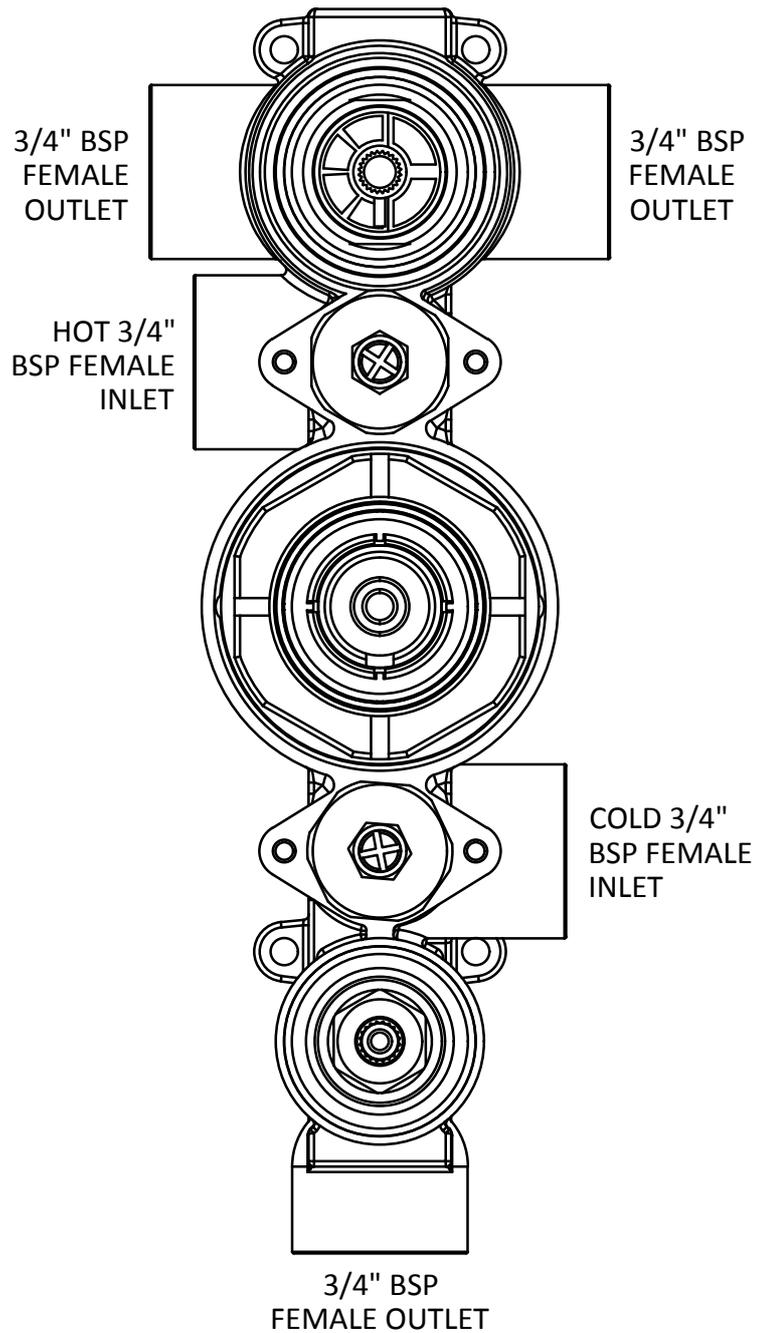
**Twin Valve with Diverter**
