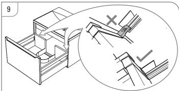
When re-fixing the drawer back to the runners, ensure that they click into position on both sides and the back of the runner is flush with the back of the drawer on both sides (see Fig.9).
