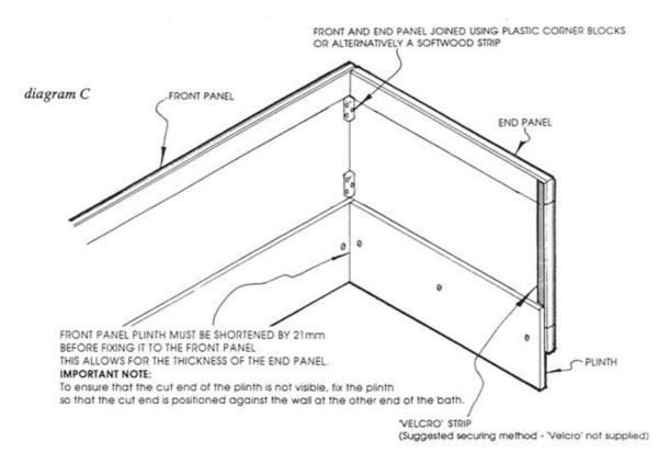
Once the front and end panels are joined together the assembly can be secured at each "loose" end to the softwood strips. (see diagram D).
