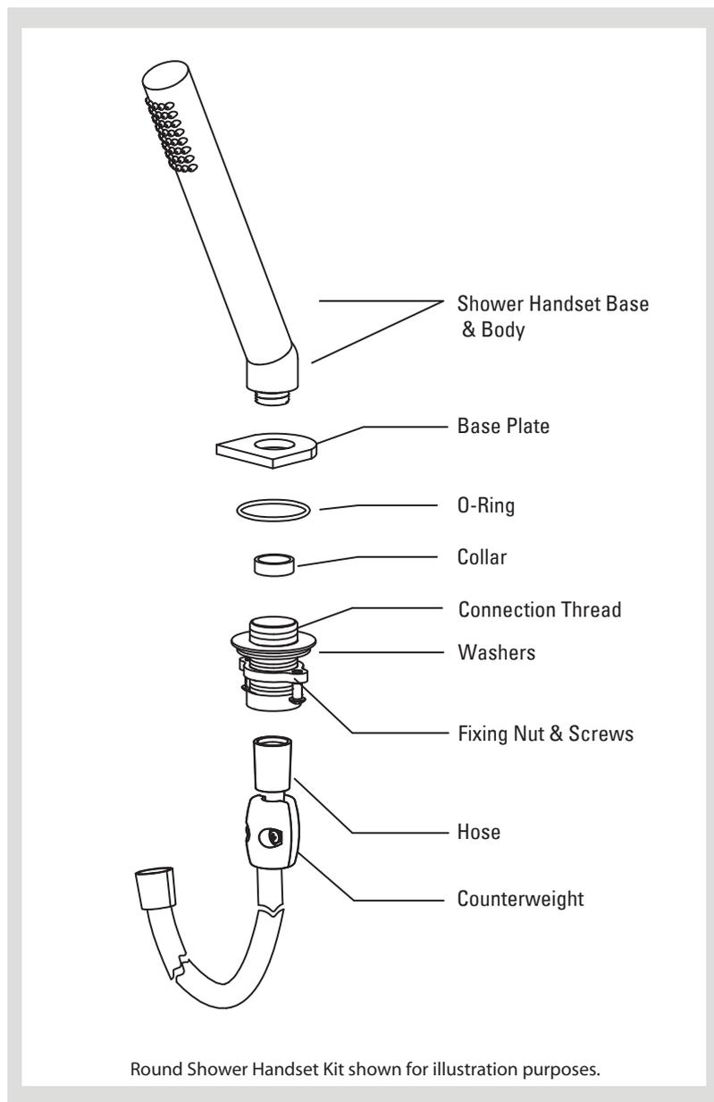
1. Attach the counter weight to the shower hose, allowing enough room for the hose to be retracted to an appropriate length later.
